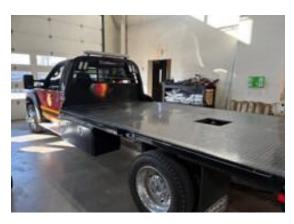
The 2012 chassis was then repurposed by installing a flatbed unit and a snow plow to serve as a utility vehicle for District facilities.
